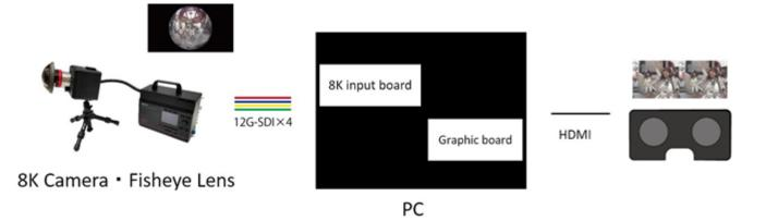
Real-time live stereo VR live using two 8K cameras. By combining with the fisheye lens, we shoot 8KVR video with high resolution and without stitching.
