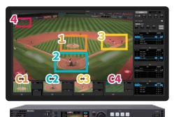
Extracts four separate 1080/50P videos from 4K/8K input/footage, virtually controlling multiple cameras with a single device
